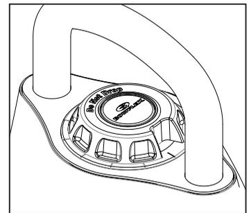
**!** Do not use too much force to try to turn the locked adjustment knob. Too much force can damage the locking mechanism.
